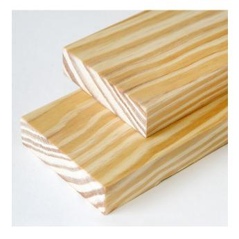
After trees are harvested, they are sawn into boards and dried in a kiln. This lowers the moisture content, stabilizes the board and increases its strength.
